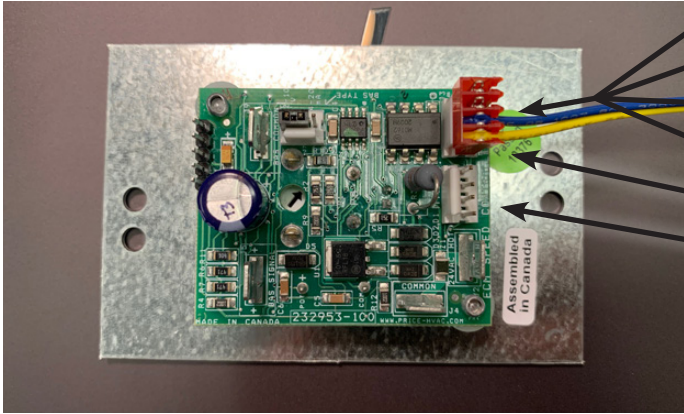
FIGURE 6 - ECM STANDARD SPEED CONTROLLER - CONTROL CABLE PINOUT ▼
